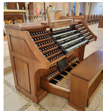
The terraced console features four manuals and turned African Blackwood drawknobs with faux ivory engraved inserts.
