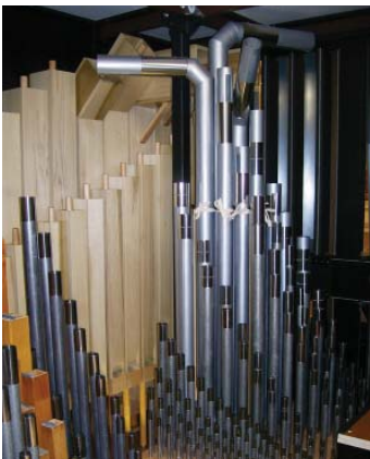
Mitered pipes in the Swell chamber (photo credit: Patty Conley)
